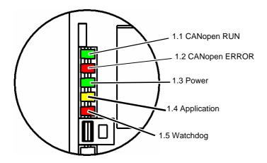
The "Controller Inside" card is equipped with five LEDs which can be seen through the window in the Altivar 61 / 71 cover.
