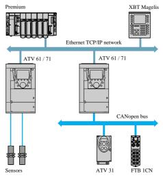
Modular machine with Ethernet TCP/IP network
