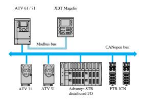
The master CANopen port on the "Controller Inside" programmable card can be used to extend the I/O capacity (using CANopen I/O modules) and to control other CANopen slave devices.
