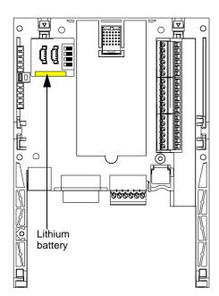
When installing the "Controller Inside" card in the drive, make sure that this battery is present. It takes the form of a rectangular block clipped onto the non-volatile RAM (see schematic opposite).
