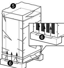
7. Lift up the cabinet with a forklift and remove the two pieces of plywood.
