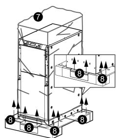
9. Lift up the cabinet with a forklift and remove the two pieces of plywood.
