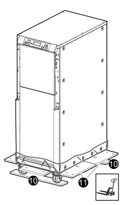
12. Remove the plastic film, cut the strappings around the casters, and roll down the cabinet from the two pieces of plywood.
