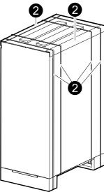
3. Remove the two top plywood plates and the cardboard box.
