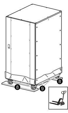
10. Remove the plastic film, cut the strappings around the casters, and roll down the cabinet from the two pieces of plywood.
